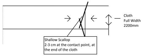
Material should be hemmed first then squared. Undercut if necessary the spline line with a shallow scallop ready to mount on the roller.
